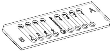
The ibidi product family is comprised of a variety of  $\mu$ -Slides and  $\mu$ -Dishes, which have all been designed for high-end microscopic analysis of fixed or living cells. The high optical quality of the material is similar to that of glass, so you can perform all kinds of fluorescence experiments with uncompromised resolution and choice of wavelength.
