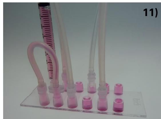
**Bend the Serial Connector and adapt the free male Luer adapter to the neighboring Luer port on the slide. Take care not to trap an air bubble in the Luer port!**
