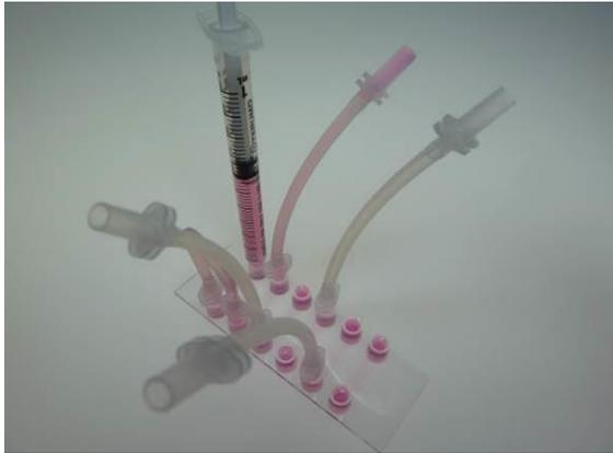
Now repeat the last four steps for every new connection. First fill the next Serial Connector with medium...
