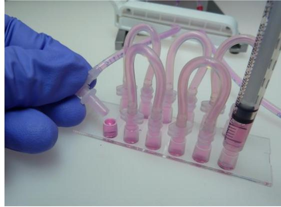
**Pull the male Luer connector out of the Female Luer Lock Coupler of the Perfusion Set and place it into the remaining Luer port on the slide. Now slowly pull out the syringe and fill the Luer port to the top with fresh medium and remove the air bubbles.**
