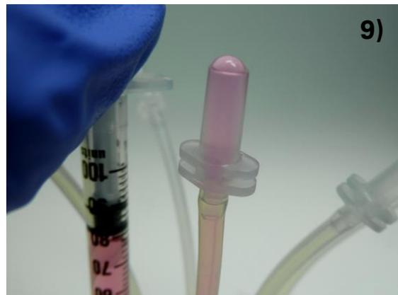
**Slowly push the medium through the channel and the first serial connector until the medium fills the Luer connector completely**
