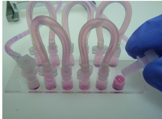
**After removing the syringe, pull the second male Luer connector out of the Female Luer Lock Coupler of the Perfusion Set and place it into the remaining Luer port on the slide.**
