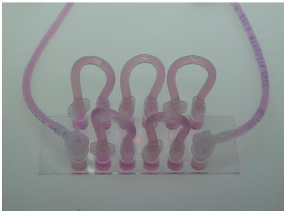
**The setup is finished and ready for starting the flow. Don't forget to remove the hose clip!**
