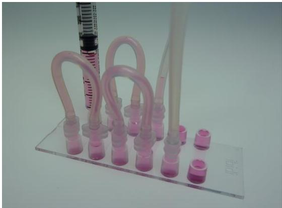
Three Serial Connectors are connected.
