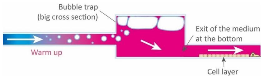
**Figure 3 Principle of a bubble trap**
