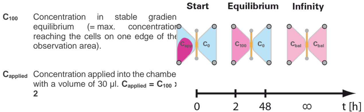
$C_{balanced}$  Balanced chemoattractant concentration after an infinite time calculated with the total chamber volume of 130  $\mu$ l.
