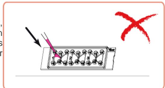
**Avoid trapping air by filling empty reservoirs with the  $\mu$ -Slide inclined. Always inject the liquid into the lower reservoir in order to allow the lighter air to escape on the top.**
