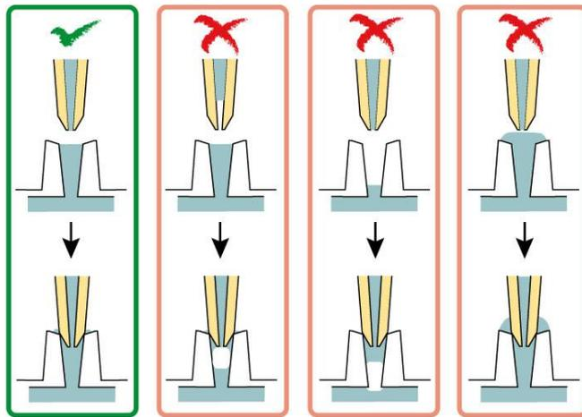
**Avoid unfilled filling ports and air bubbles inside the pipet tip!**
